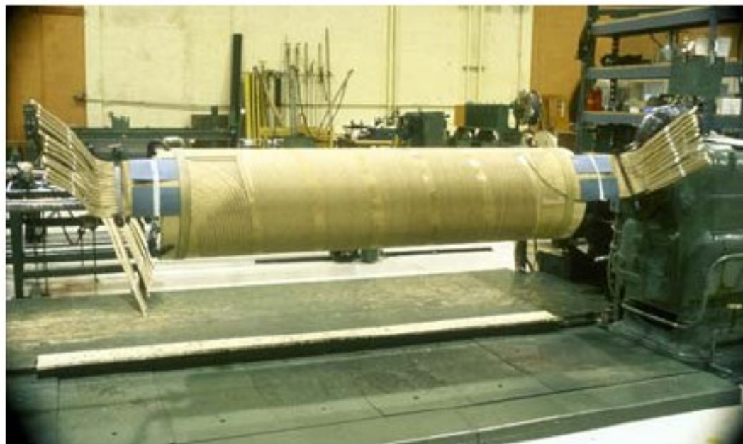
Regulating Voltage Winding Design
